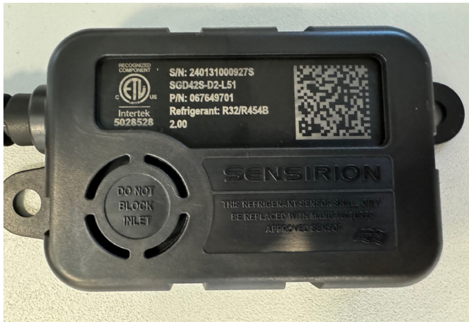
FIGURE 7. Example of Clear, Unobstructed Sensor Inlet
